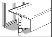
7. Connect the bath drain to the drain pipe. Position a protective liner in the bath basin.
